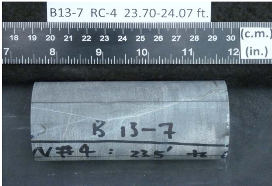
After cutting and grinding
